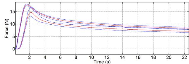
Fig. 7: Force exertion experiments for a two-phalanges robot finger at two different configurations (30% and 70% flexed). For each configuration, multiple experiments were conducted. The red lines represent the mean values and the blue dotted lines the min and max values per configuration. The high forces values correspond to the 30% flexed case and reach 18 N (peak), with a standard servo.
