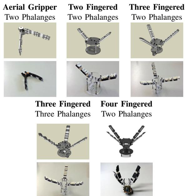
Fig. 8: Different robot hand models and robot hands created with the design directions provided, are depicted.
